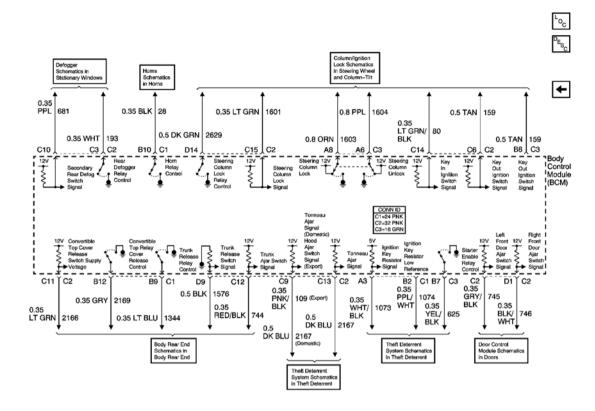
Fig. 3: Subsystem References Schematic Courtesy of GENERAL MOTORS CORP.
