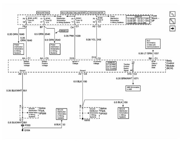
Fig. 1: Power, Ground, and DLC Schematic Courtesy of GENERAL MOTORS CORP.
