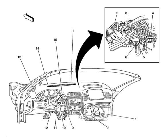
Fig. 4: Instrument Panel Component View Courtesy of GENERAL MOTORS CORP.
