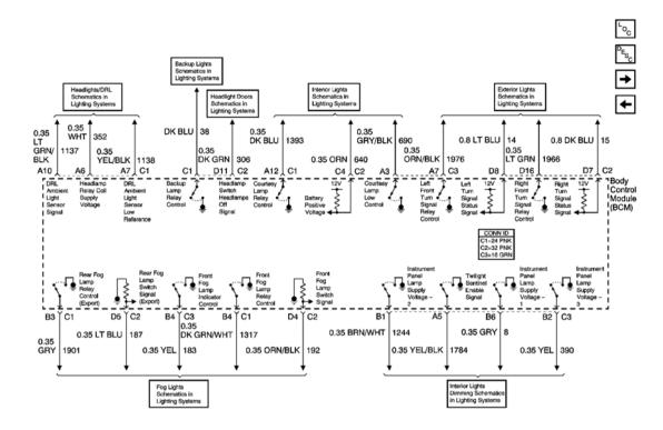
Fig. 2: Lighting References Schematic Courtesy of GENERAL MOTORS CORP.
